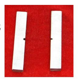
**U5** type (ISO148, GB/T229, Gost 9454) and Type C (ASTM E23), non-standard type, short using life, no warranty
